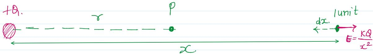
$\therefore$  small work done to move the unit +ve charge by a small dist  $dx$
