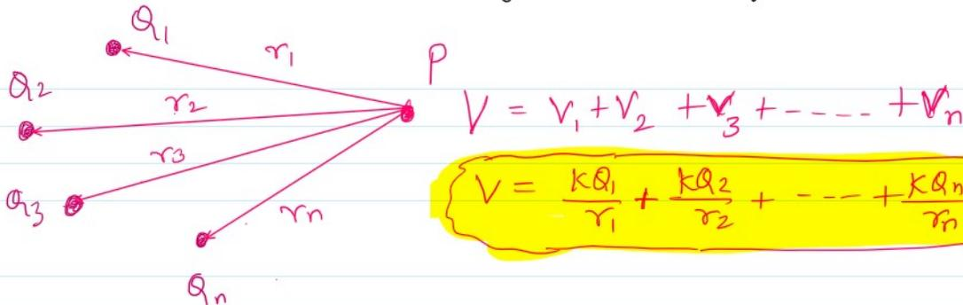
$$V = \frac{kQ_1}{r_1} + \frac{kQ_2}{r_2} + \dots + \frac{kQ_n}{r_n}$$
