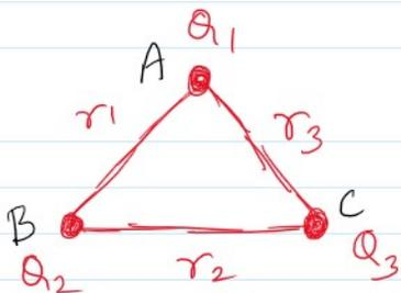
$$PES = 0 + \frac{kQ_1 \times Q_2}{r_1} + \frac{kQ_1 \times Q_3}{r_3} + \frac{kQ_2 \times Q_3}{r_2}$$
