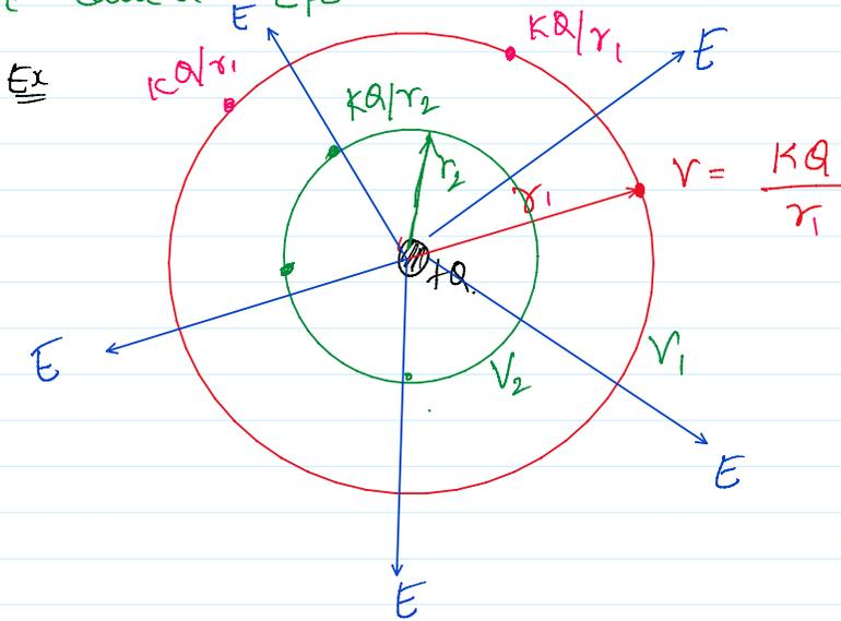
The shape of EPS is spherical due to point charge.
